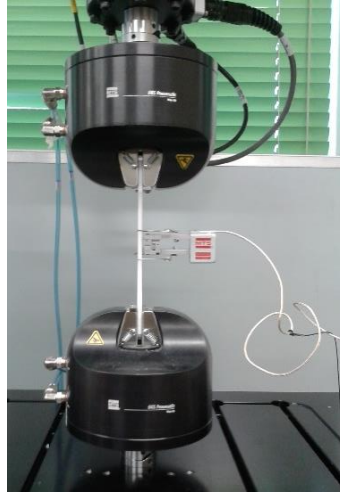
Figure 102. Tensile test setup. ISO 527 type 1A sample produced by SLS technology gripped by the MTS Acumen 3 Electrodynamic Test System and with the extensometer connected.
