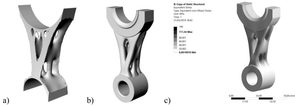
Figure 8. Topology optimization model: a) SOLIDWORKS® Simulation result, b) remodeled part in Altair Evolve, c) equivalent Von-Mises stress.
