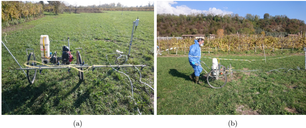
Figure 2.4: Application of the solution containing the tracer and the glyphosate-based herbicide. (a) The tool used for the application of the solution featuring the concentrations listed in Table 2.3. (b) The application of the solution.
