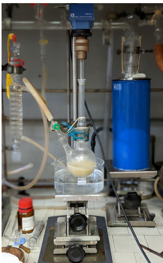
Figure 3.2: Mechanical stirring system used for the preparation of the epoxy/clay nanocomposites. The flask containing the reacting mixture was connected to a high vacuum pump system and was cooled by an external bath of cold water.
