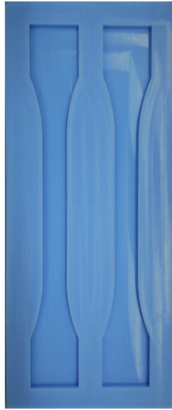
Figure 3.3: Dog-bone (DB) shaped silicon rubber moulds used for the production of the epoxy/clay nanocomposite samples.
