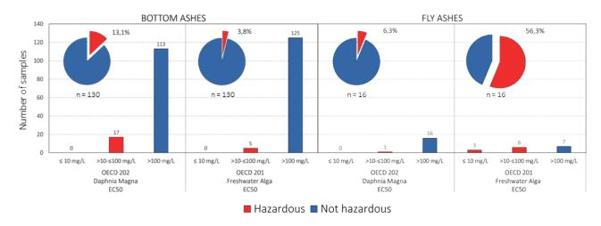
FIGURE 1: Results from the ecotoxicological tests (i.e., the "direct" approach) applied to samples of BA (n = 130 samples) and FA (n = 16 samples), already classified as hazardous for HP 14 by measured substances concentration (i.e., by the "indirect" approach).
