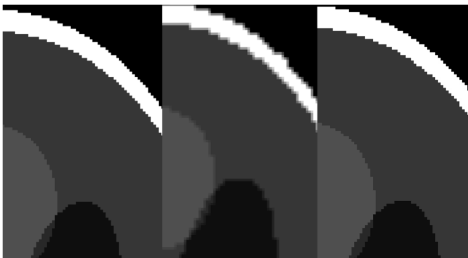
Fig. 3. Left: a zoom of an axial slice of the high resolution Shepp–Logan phantom. Center: the same slice oversampled with Trilinear interpolation. Right: the same slice oversampled with Trilinear interpolation and Fake Nodes.
