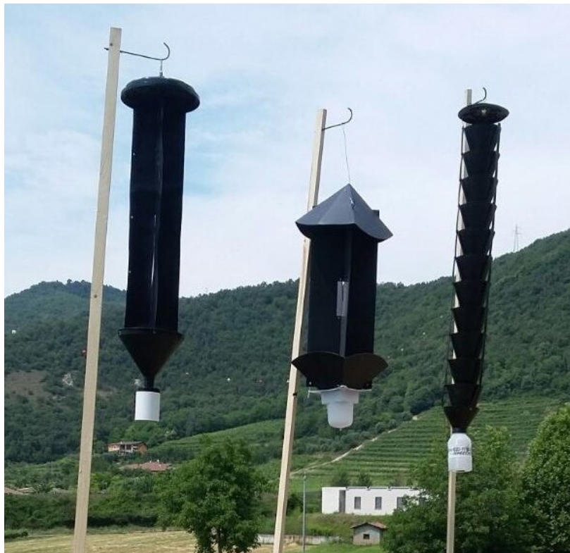
Fig. 2 The traps used in this study. From left to right: soft cross-vane (Econex), standard cross-vane (Witasek), multi-funnels (Witasek) on the support wooden poles.
