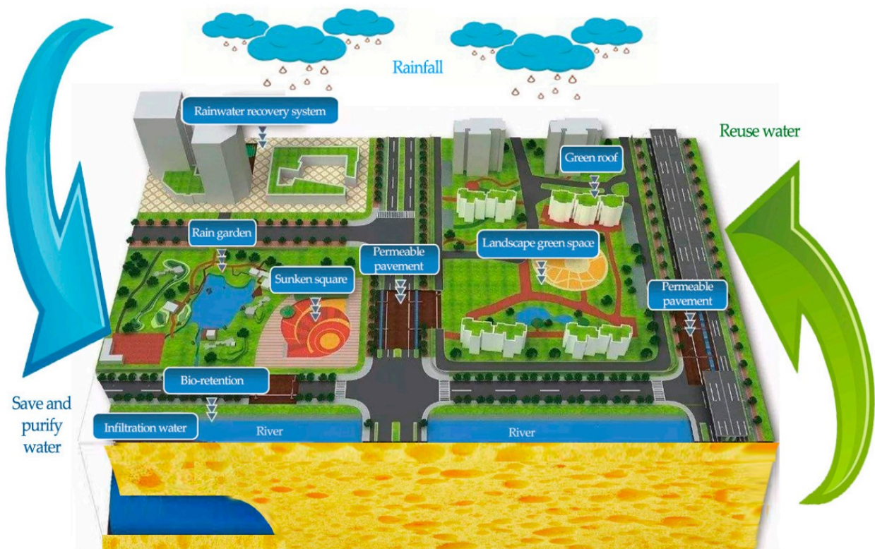
Figure 1-12 Schematic diagram of the sponge city concept. (Source: Chen and Chen, 2020)
