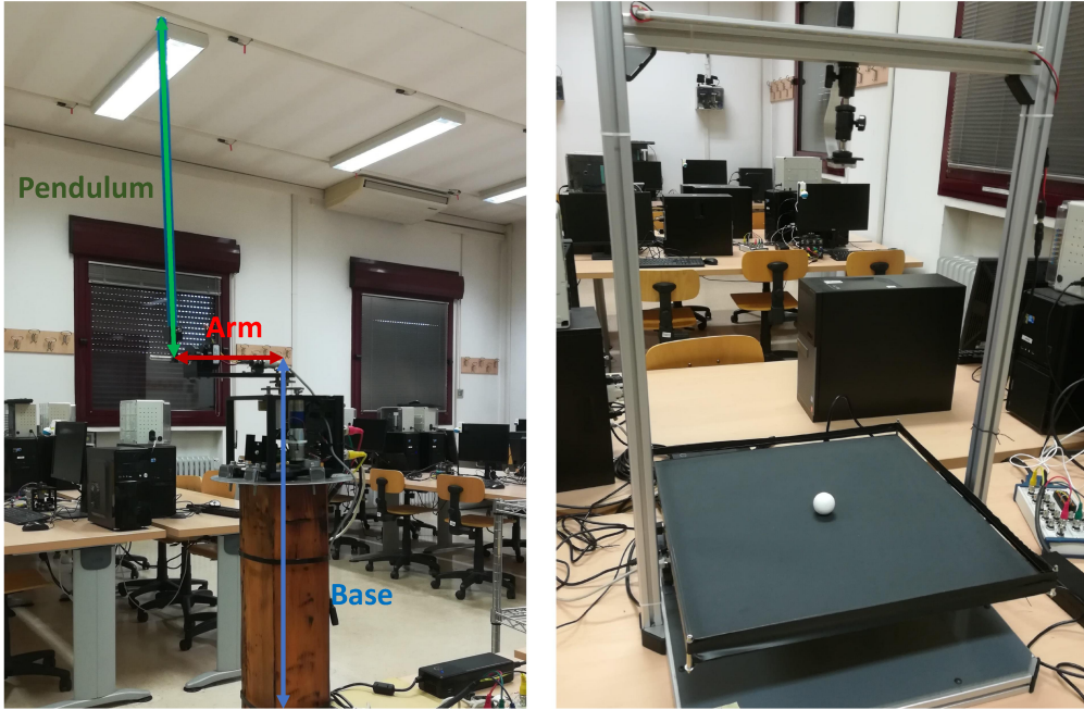
Figure 3.4: (Left) Furuta pendulum used in the experiment while being controlled in the upward equilibrium point by the learned policy. (Right) Ball-and-plate system.
