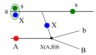
**Fig. 10** A schematic description of the Trojan horse method. The projectile nucleus a consists of two fragments, X and s, for which the fragments X fuses with the target nucleus A while the fragment s acts as a spectator. After X fuses with A, the compound nucleus decays into B+b
