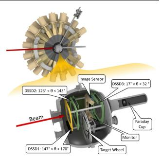
Fig. 8 Schematic of the experimental setup at ANL for the first particle- $\gamma$  coincidence measurement at astrophysical energies. The spherical target chamber is mounted in the middle of the Gammasphere array [55,56]
