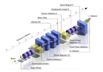
Fig. 6 The velocity filter SHIP, installed at GSI [42,43]
