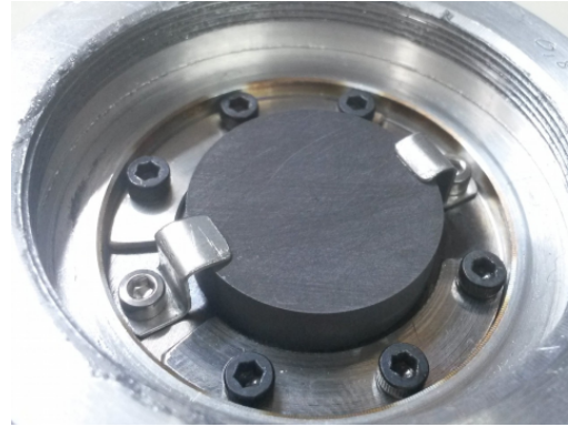
Figure 2.4: The picture of the graphite disk mounted on the target holder. The disk is placed on a blank Ta disk of the same thickness as in the evaporated target case.
