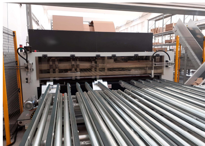
Figure 5. The new die-cutting machine (Case 1—own research).
