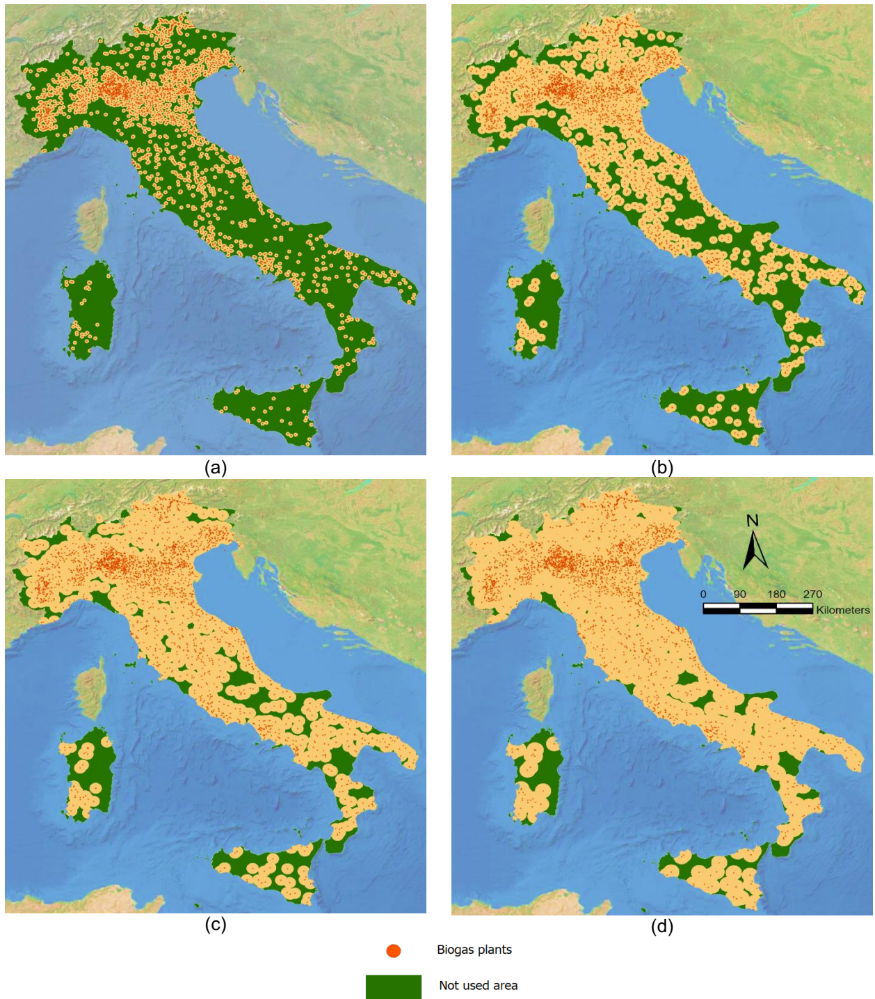
Figure 3-6. Biogas plants and unused areas in 5 km (a), 10 km (b), 15 km (c) and 20 km (d) radii
