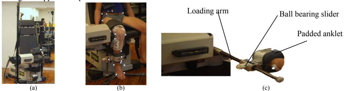
Fig. 1. (a) Technogym REV 7000 isokinetic machine; (b) subject equipped with reflective markers for testing; (c) detail of the loading arm with a ball bearing slider
