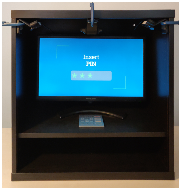
Figure 3.3: Our experimental setup. The cameras are visible but they can be hidden into the frame of an ATM. In all other aspects, we reproduced a common ATM layout in detail.
