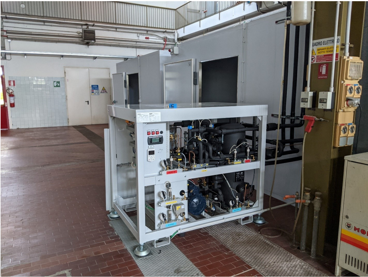
Figure 4.3 – R744 cooling unit experimental setup, installed at ITC-CNR laboratories.
