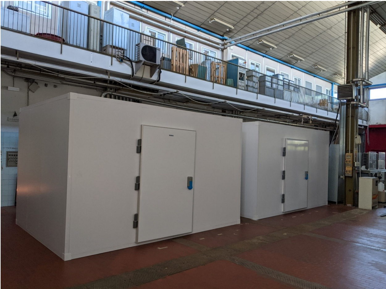
Figure 4.5 – Insulated chambers in which the heat exchangers are placed, to reproduce the desired heat sink and heat source temperatures during experimental tests.
