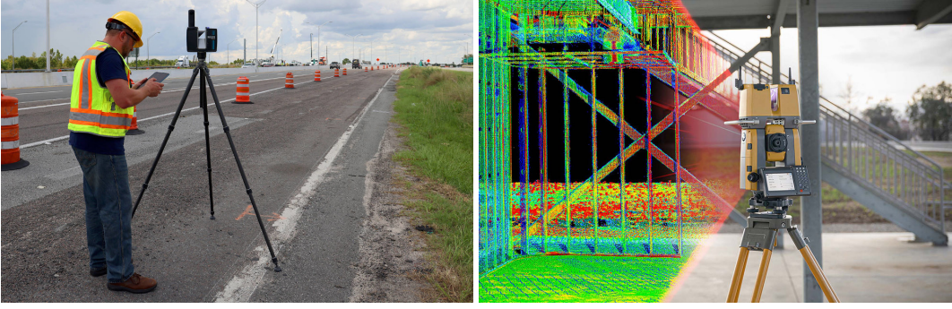
FIGURE 2.7: Two examples of terrestrial laser scanners (TLS): a FARO ® scanner (left) and a Topcon ® GTL-1200 (right) (Courtesy of FARO ® and Topcon ® ).
