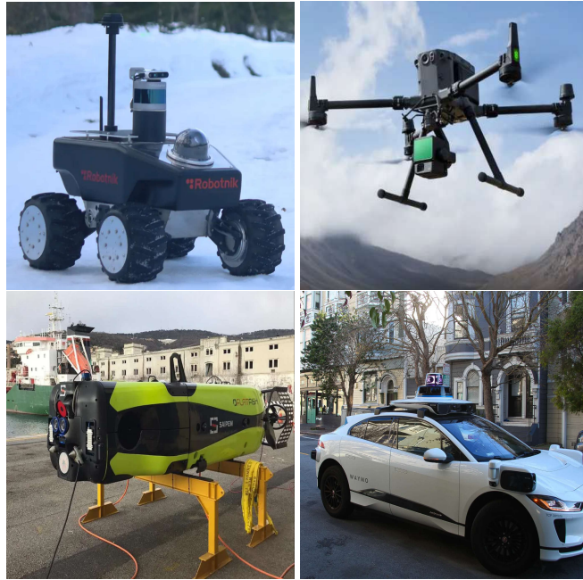
FIGURE 1.1: At the top, from left to right, are an unmanned ground vehicle (UGV) with manipulator ( Courtesy of Robotnik ), an autonomous underwater vehicle (AUV) (FlatFish, Courtesy of Saipem ). Below are, from left to right, an unmanned aerial vehicle (UAV) ( Courtesy of DJI ) and an autonomous electric vehicle (AEV) ( Courtesy of Waymo ), serving as a robotaxi in San Francisco.
