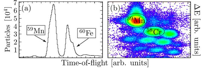
FIG. 1. (Color online) Particle identification for the  $^{58}\text{Cr}$  setting. (a) Particles of the secondary beams are identified by means of a time-of-flight measurement. (b) Reacted beam particles are identified by their energy loss  $\Delta E$  in the ionization chamber and their time-of-flight through S800 (incoming particle gate is set on  $^{59}\text{Mn}$ ).
