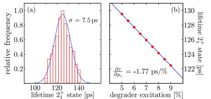
FIG. 10. (Color online) The error analysis applied to the  $2_1^+ \rightarrow 0_1^+$  transition in  $^{62}\text{Cr}$ . (a) Analysis of the statistical error  $\Delta \tau_i$ . (b) Influence of degrader excitation on the deduced lifetime. Simulated data is shown in red (light gray) while fits are shown in blue (dark gray).
