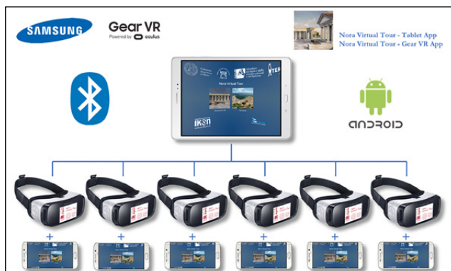
Fig. 3 – Schematic representation of the Nora Virtual Tour system.
