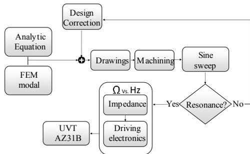
Figure 2. Workflow of the design procedure.
