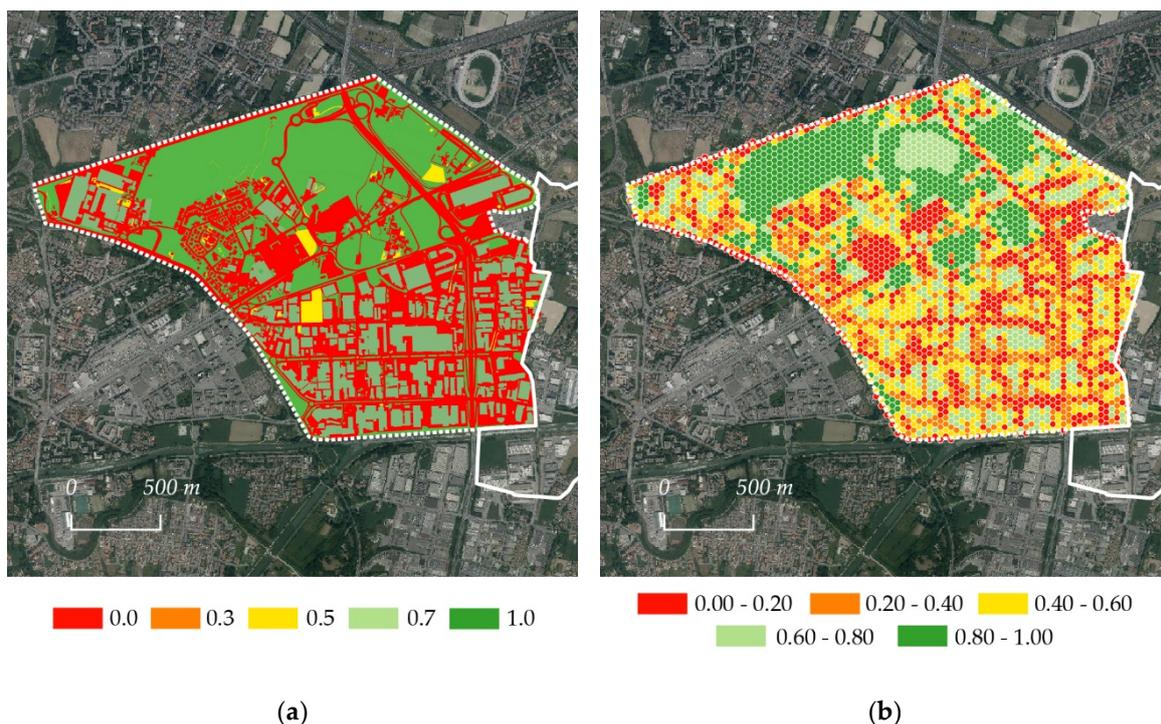
**Figure 10.** Mitigation scenario in the San Lazzaro neighborhood: rooftop greening. (a) BAF analysis showing different degrees of permeability (from 0 to 1); (b) Hexagon tessellation of the BAF analysis.
