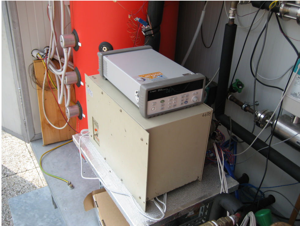
Figure 2.4. Ice point and Agilent 34970A data logger.
