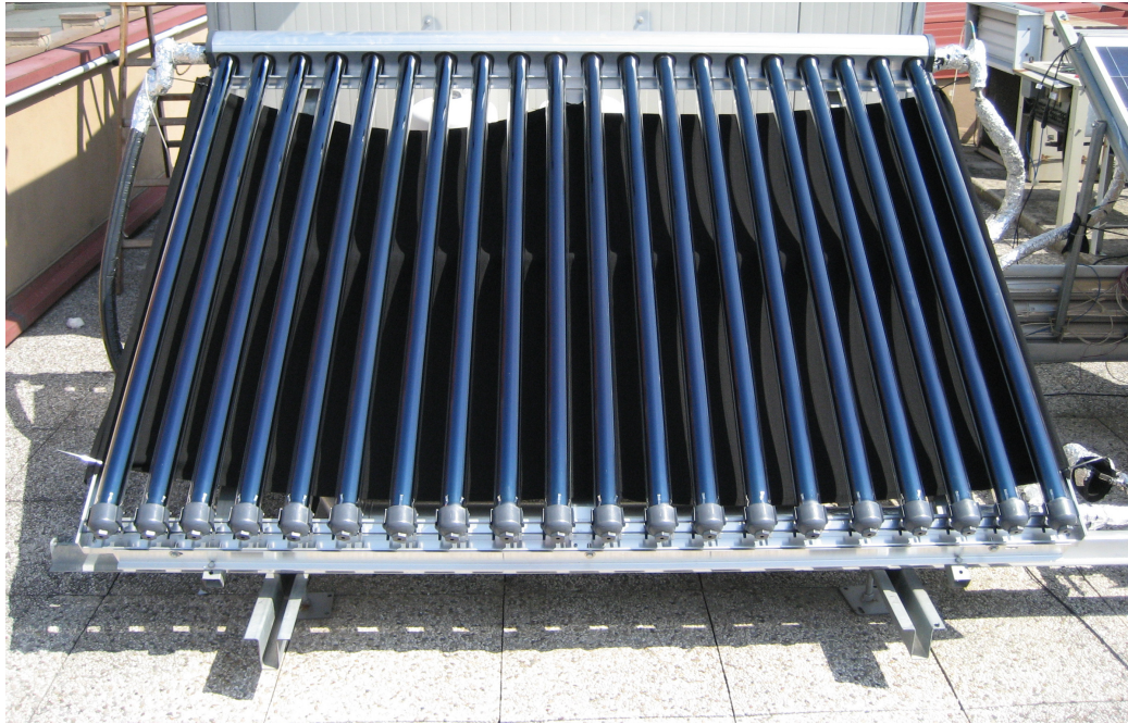
Figure 6.2. Evacuated tube collector installed in the apparatus without CPC reflectors.
