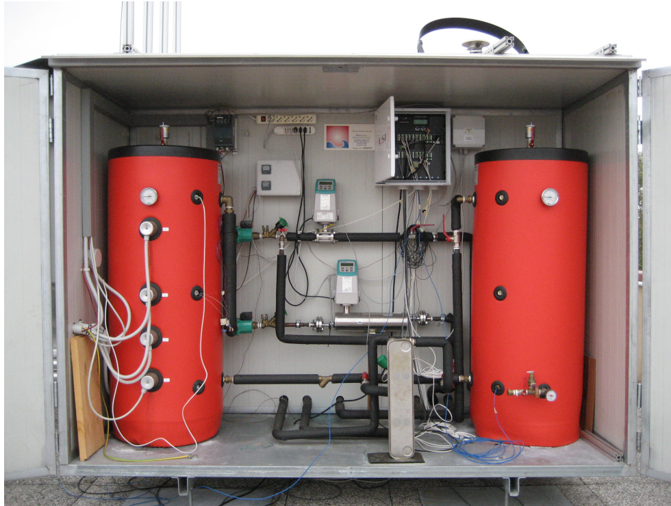
Figure 2.2. Hydraulic loop: Storages, pumps, fluid flow meters and plate heat exchanger (heat sink).
