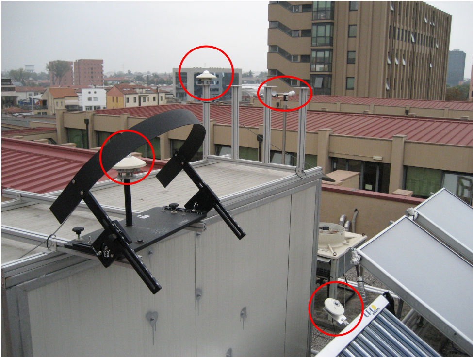
Figure 2.3. Irradiance measurements and anemometer.
