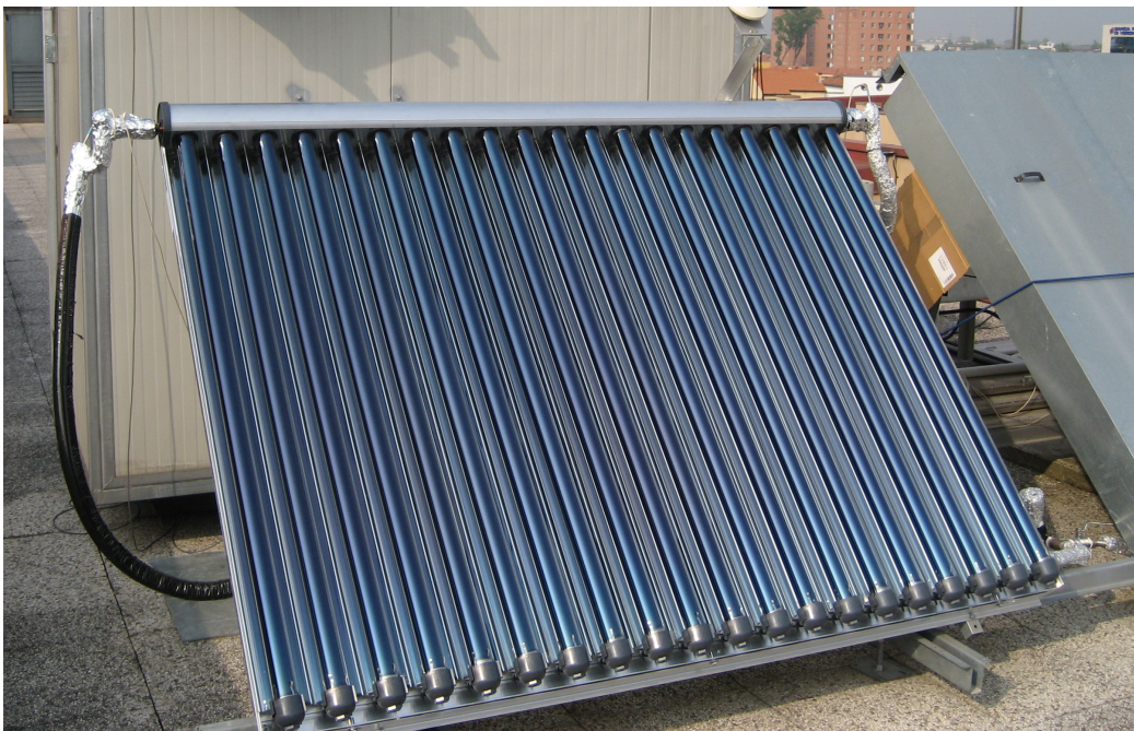
Figure 6.1. Evacuated tube collector installed in the apparatus with CPC reflectors.
