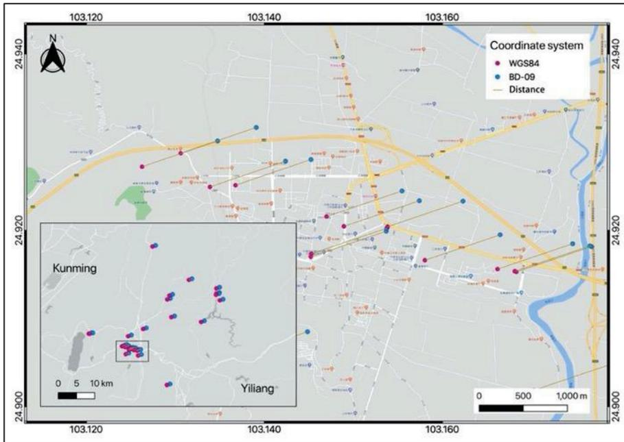
Figure 75, Offset between BD-09 and WGS 84
