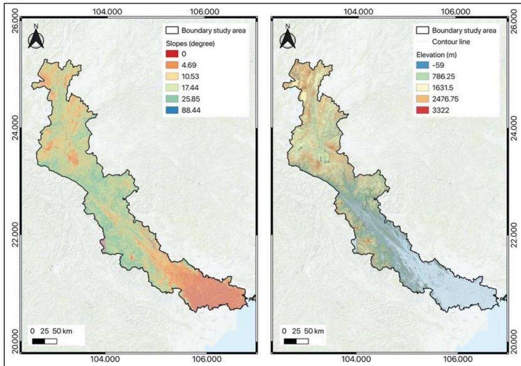
Figure 81, Result of clipped DEM in study area
