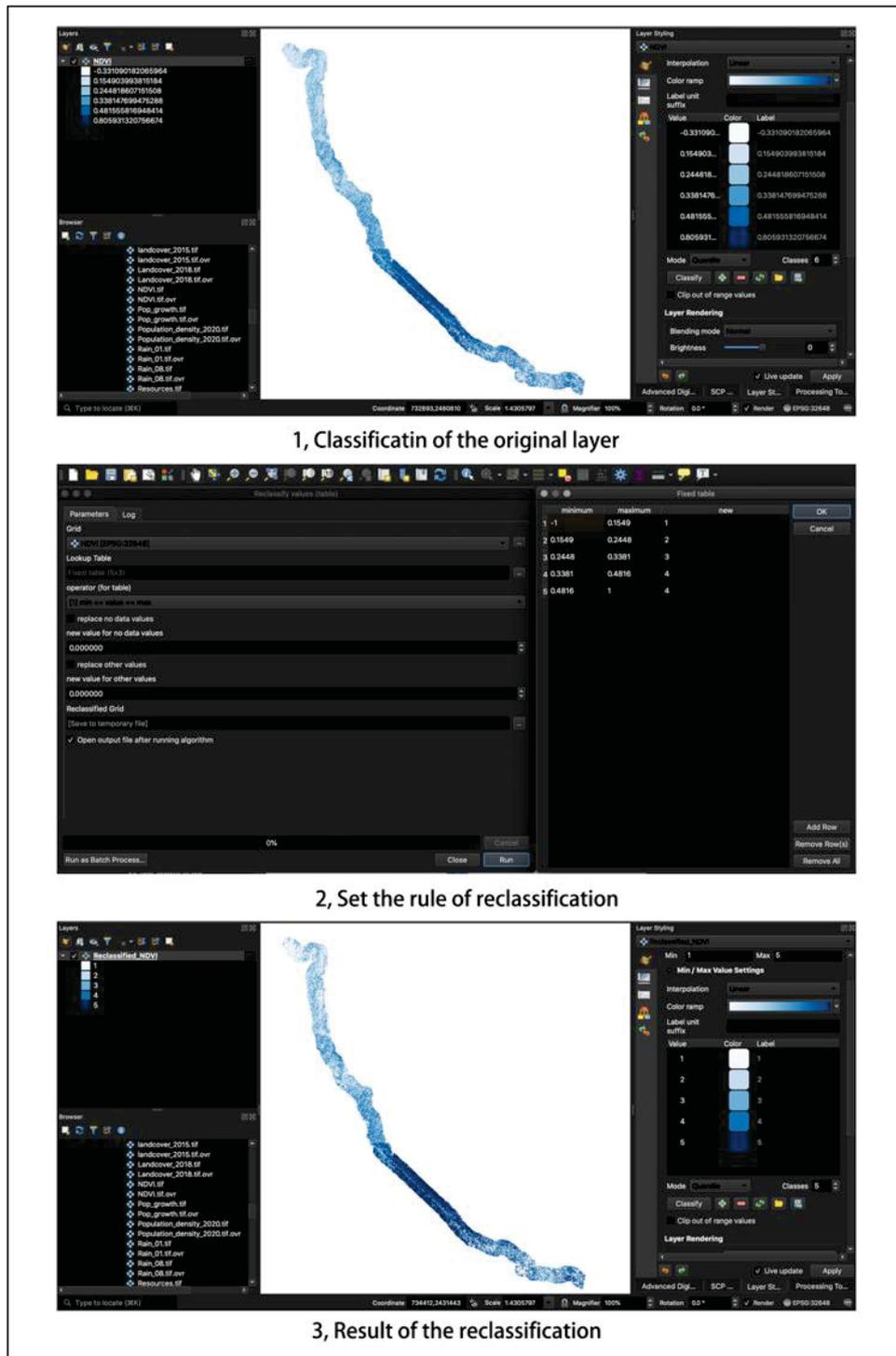
Figure 107, Reclassification of the index layer
