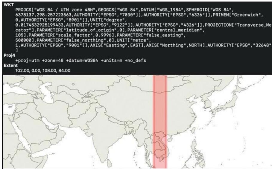
**Figure 73, Parameters of UTM zone 48N**
